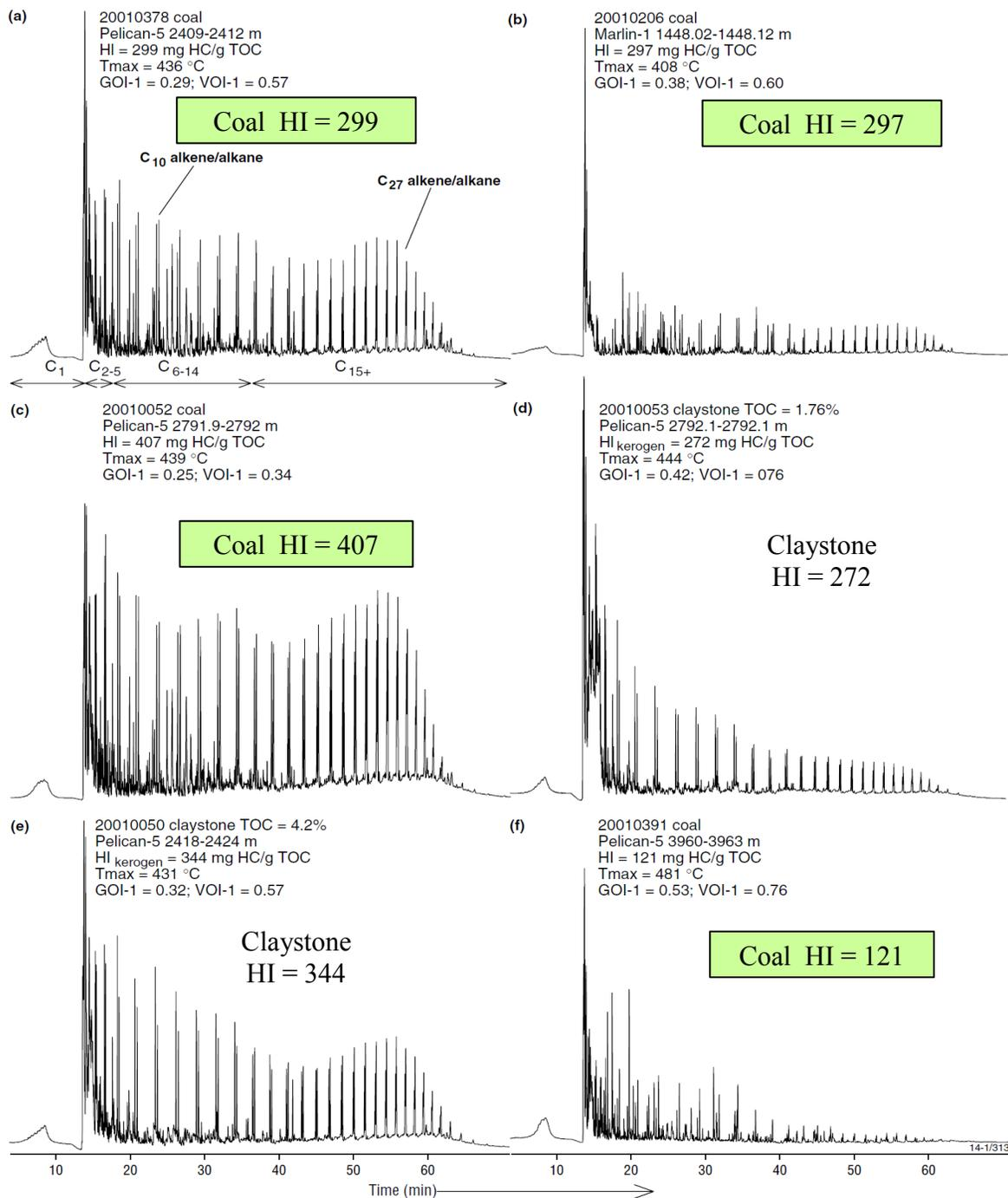
Figure 8. Py-GCMS chromatograms for coals from Pelican-5, Bass Basin; a), c), f) and Marlin-1, Gippsland Basin, b), and, claystones (kerogen) from Pelican-5, d) and e). For claystones note the slight increase in HI<sub>kerogen</sub> compared to HI for the whole rock (Table 2).
