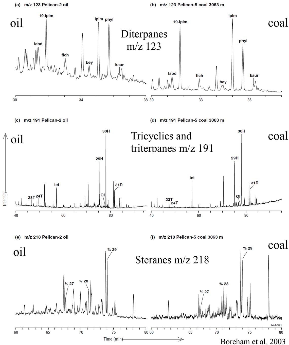
Figure 16. GCMS traces for saturated hydrocarbons for Pelican-2 oil and Pelican-5 coal from 3063 m showing a) and b), diterpanes m/z 123; c) and d), tricyclics and triterpanes m/z 191; and, e) and f), steranes m/z 218. Note: for peak identifications see Table 3.
